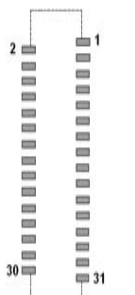
HRS/DF9C-31S-1V(22) PCB FOOTPRINT
